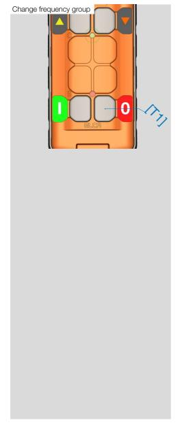
LED flashes once, then the transmitter unit switches off.
